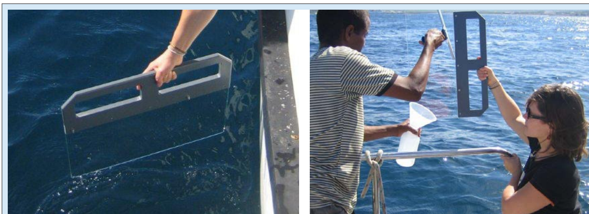
Fig. 4: (left) Sampling of the SML using the glass plate technique. (right) Collection of the SML using Teflon Wipers.
