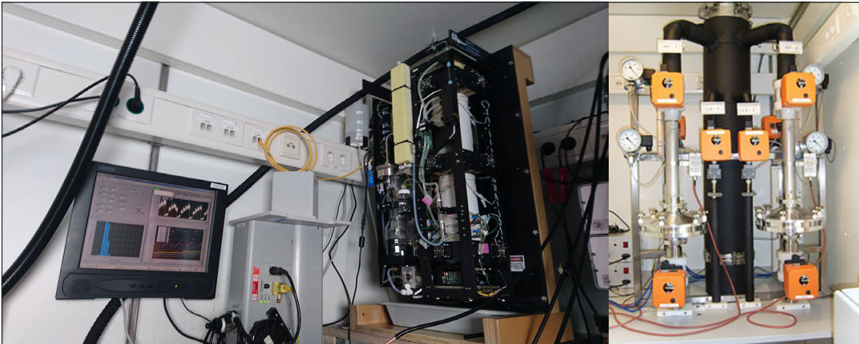
Fig. 1: CCN instrument (left) and the low volume sample set-up (right) as installed in the AWI Air Chemistry Observatory at Neumayer Station III. Both units sample from the same whole air inlet as the other aerosol instrumentation, which is situated on top of the measurement container.
