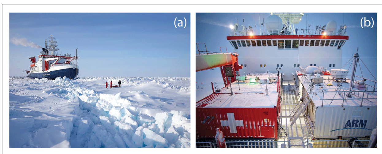
Fig. 1: The Polarstern (a) drifting in the Arctic ice on 10 April 2020 and (b) measurement containers for in situ aerosol monitoring (the first two containers on the left side and the first container on the right side) and for remote sensing of aerosols and clouds. The OCEANET-Atmosphere container of TROPOS is the third one on the left side (with the bright spot on the roof caused by green laser light). The ARM mobile facility (AMF-1) is shown on the right side. The photographs were taken by Michael Gutsche (CC-BY 4.0), AWI.
