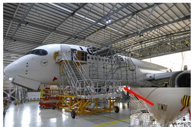
Fig. / Abb. 10: Conversion of the Lufthansa Airbus A350-900 for IAGOS-CARIBIC. / Umbau des Lufthansa-Airbus A350-900 für IAGOS-CARIBIC. (Photos: Torsten Gehrlein, KIT; Montage: Peter Braesicke, KIT; https://www.kit.edu/kit/28770.php )
