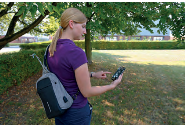
Fig. / Abb. 9: Citizens were able to research fine dust and soot in Leipzig in several field phases of the WTimpact project. Dr. Denise Assmann demonstrates the measuring backpack developed for this purpose. / Bürgerinnen und Bürger konnten in mehreren Feldphasen des Projekts WTimpact Feinstaub und Ruß in Leipzig erforschen. Dr. Denise Assmann demonstriert den dafür entwickelten Messrucksack. (Photo: Tilo Arnholt / TROPOS)
