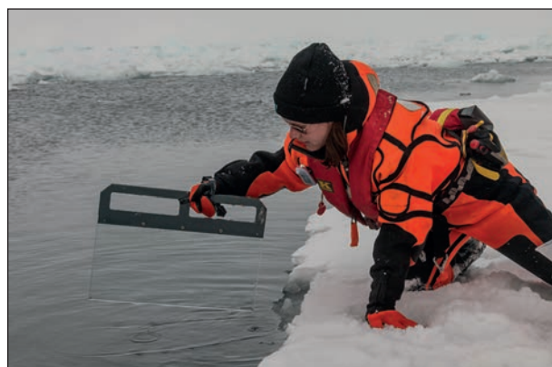
Fig. 10: Surface microlayer (SML) sampling at the ice edge. Picture by Marcel Nicolaus, AWI.
