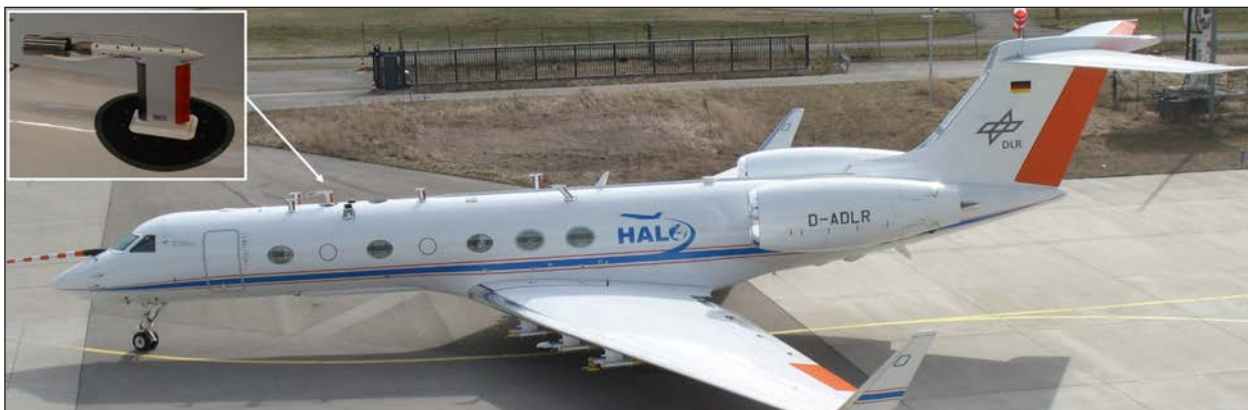
Fig. 1: Inlets and wing probes installed at the German research aircraft HALO for the ML-CIRRUS mission. The position of the HALO-CVI inlet developed by TROPOS (shown in the enlarged detail) is indicated.
