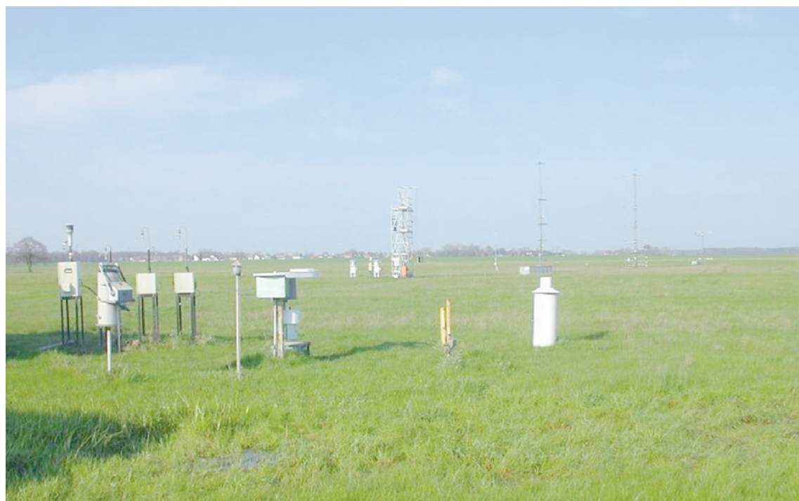
Fig. 1: Overview to west at the Melpitz site. In the foreground (right hand side) the Partisol 2000 air sampler with different impactors.
