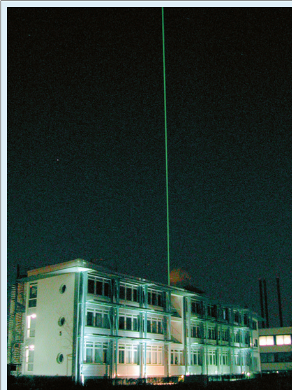
Fig. 5: Multiwavelength Raman lidar measurement after sunset performed in the framework of the European Aerosol Research Lidar Network (EARLINET).
