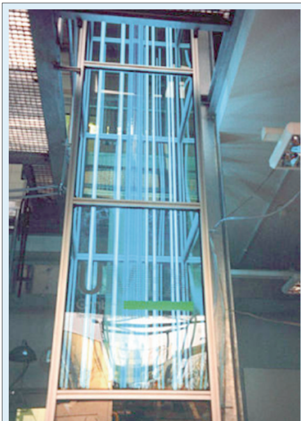
Fig. 6: The IFT laminar flow tube reactor (IFT-LFT).
